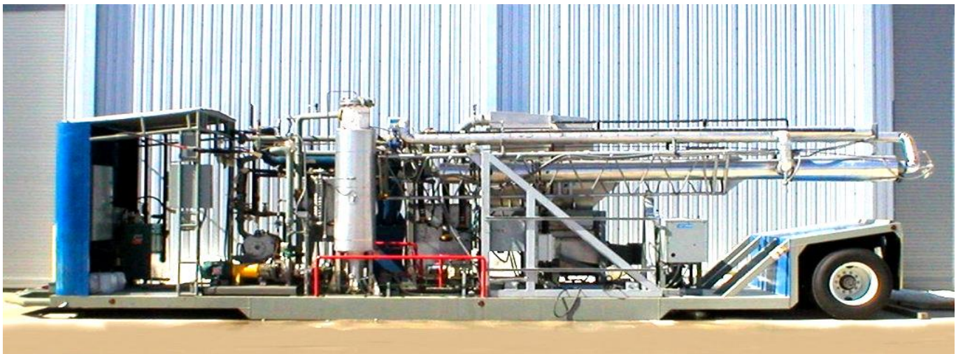
Mobile BCS with Fluidized Bed Heat Exchanger folded down for relocation
