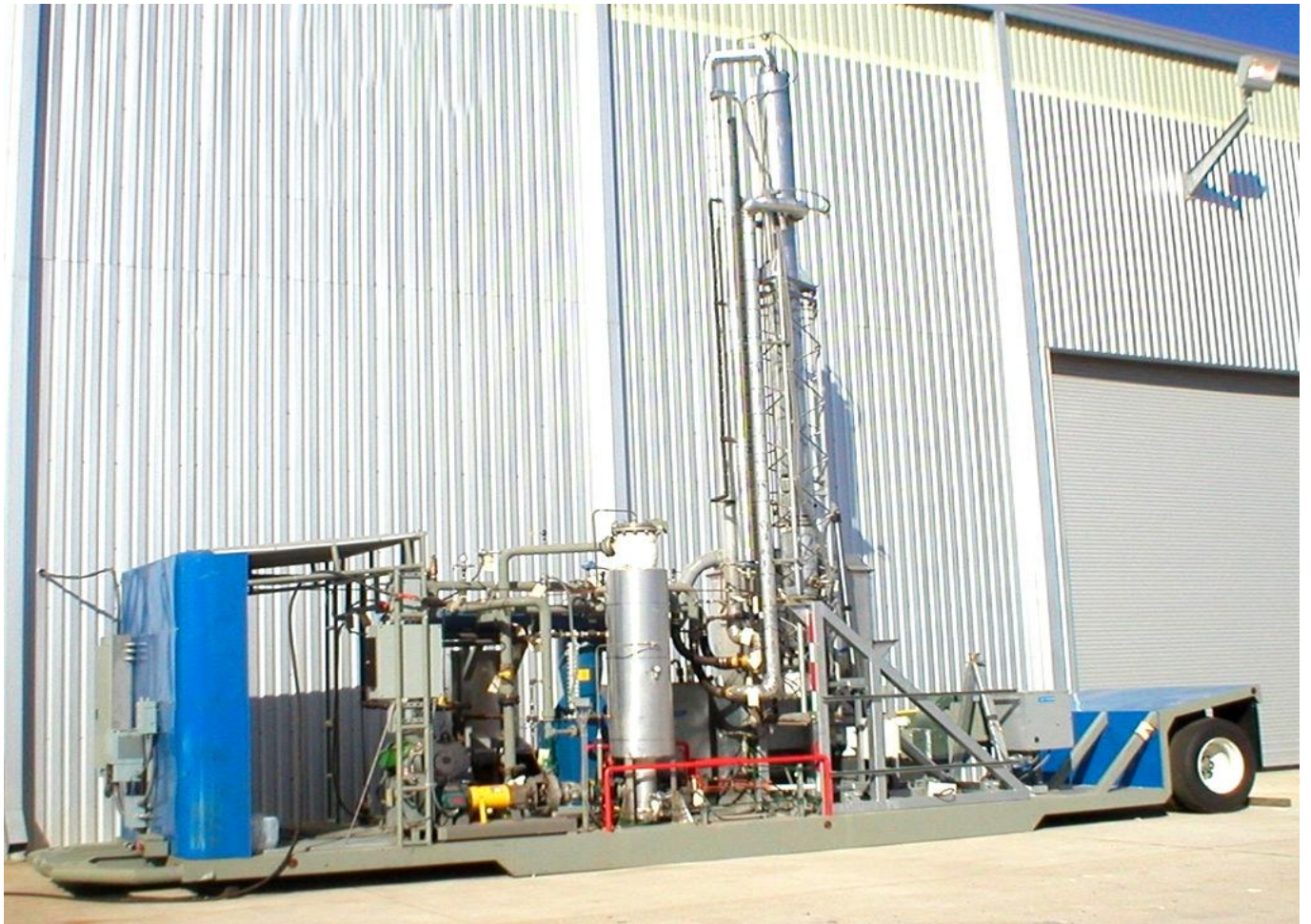
50 barrel per day Brine Concentrator System (BCS) Test / Demonstration Unit
